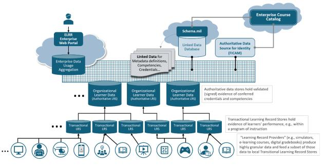
**Figure 5. Enterprise Digital Learning Data Fabric.** *The TLA's federated data structures maintain data ownership with local DoD components while ensuring all data is accessible by other connected systems.*
